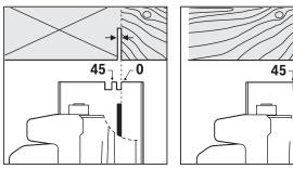
The 0° cutting mark 10 indicates the position of the saw blade for right-angled cuts. The  $45^\circ$  cutting mark 9 indicates the position of the saw blade for  $45^\circ$  cuts.
